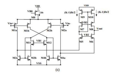
Figure 1.1. (a) Folded cascode OTA (b) Telescopic OTA (c) Recycling Folded Cascode OTA In applications where speed, signal headroom and noise are of significance, the Folded Cascode OTA is most suited, all things being considered. It comes as no surprise therefore, to see the Folded Cascode amplifier being increasingly used either as a single stage, or as the first stage amplifier in a multi-stage amplifier, in the leading-edge designs as well as in literature [42].
